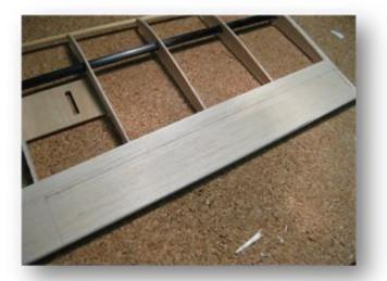
Mark with a ruler the later ailerons. They should 35 mm deeply its and shortly before the fourth rib end (see picture).
