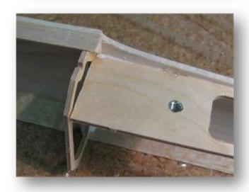
Stick now between the two side parts the head frame as well as the surface edition with Weißleim. Make sure that the surface edition is bonded correctly around and the nuts not beyond the trunk edge to stand.
