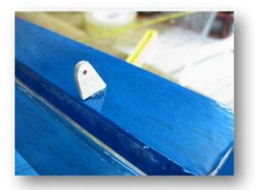
The rudders become with one strip each Tesa film from downside and above (in the order!) to the wing scharniert. In the place, to which the rudder horn is to be fastened, bore a 3 mm hole, fill this with 5 minutes of Epoxy and fix you the rudder horn.
