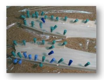
Begin to strengthen the two trunk halves at the ground and within the range of the hood cutout with the triangle border. Within the range of the hood cutout you manufacture two borders, which into shape-sharpen you properly matching due to the large bend. The canopy is likewise stuck together on the triangle border (not however with the side part). For the gluing I recommend express wood glue.
