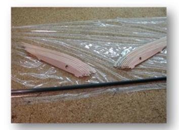
Sort the ribs of the size after and thread you these successively on the coal pipe up.
