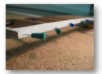
After the rudder cutout with a sharpening slat became polished straight, this is verkastet with a 1.5 mm of Balsastreifen.
