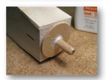
Stick now the 8 mm pegs into the sharpening template (41 mm in diameter). To hardening you put the peg into the engine frame. Thus receives equal to template the correct engine fall/course. Note! The template in no case with the trunk stick together. This serves afterwards only to sharpening the fuselage nose beautifully approximately.
