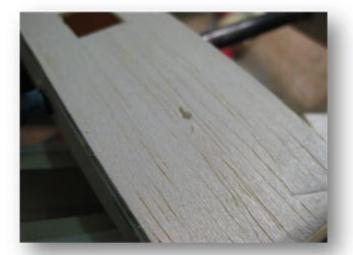
If you press now those suitably sanded bearing area on the trunk, receive a small notch in the places, in which they must 5 mm a drilling for the bearing area screw connection make.
