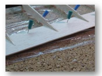
Cut the 1.5mm off Brettchen on approx. 520mm. Subsequently, you halve the two Brettchen in the center (full length), so that you receive 4 Brettchen A 520x50. End rails in such a way provide first rib for rib from downside with second adhesive on the ribs are stuck.
