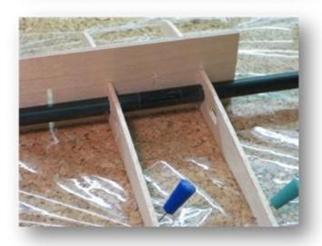
Mark the center of the coal pipe. By means of the rib comb these 40 mm are centrically arranged apart and stuck together with second adhesive.
