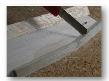
In the place, in which the canopy is to be cut out later, perforate the triangle border with a thin drill or a sharp measurer. Note: Triangle border do not split!
