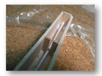
The two frames are suitably in-lived together with a bowden cable tube. The tube serves later for the inlet of the antenna cable.
