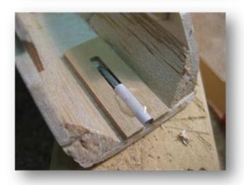
Bend they the wire around 90° and stick you it with a drop second adhesive on the plywood strip already glued to.
