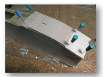
Before and behind the canopy Brettchen from the 3 mm Balsaresten are suitably cut and glued on. Do not stick the face together of the Brettchen and the canopy!
