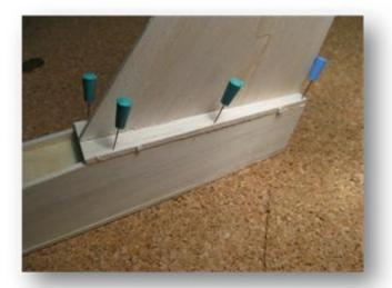
Now the rear trunk cover can be glued on. The tongue of the stuck fin can serve as guidance. The fin is however only bonded after sanding and Bebügeln.
