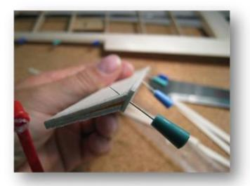
Box it the front edge of the rudders likewise with a 1.5 mm of Balsastreifen.
