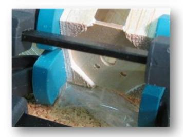
After that head frame and the surface edition drained, stick the engine frame. For this Expoxyharz is suitable. In order to receive an engine course, you leave the frame at the right trunk side approx.
