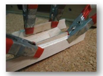
Stick the two plywood strips as guidance on the right and the left hood side as well as a further strip on the point of the hood.
