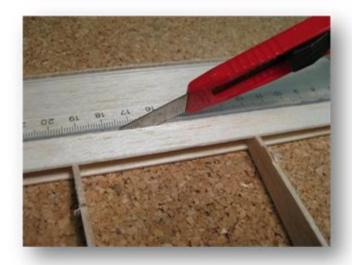
With a sharp measurer you separate now from both sides the rudders out. Mark the rudders as well as the upper/lower surface!
