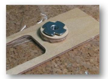
For the surface attachment you stick now the two plywood rings up and drive you with a hammer the two impact nuts. The nuts can become additionally with Expoxyharz secured.
