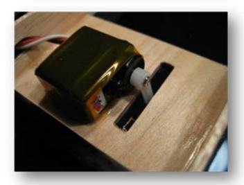
After the lower surface of the bearing area is covered with foil, the servo with a Kleks 5-Minuten-Epoxy, shrunk in heat shrink sleeve, is stuck on the servo board. On the fact it respects that the servo is in neutral position!
