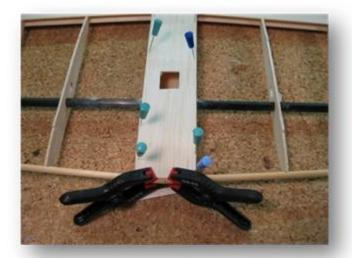
The wing center section is likewise beplankt with a remainder of the 1.5 mm of Brettchens. On the fact it respects that you cut a passage for the Servos in the center!
