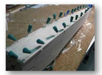
Now you can glue the trunk ground on. In addition you must grind the triangle borders at the fuselage end section, in order to receive a pointed process.
