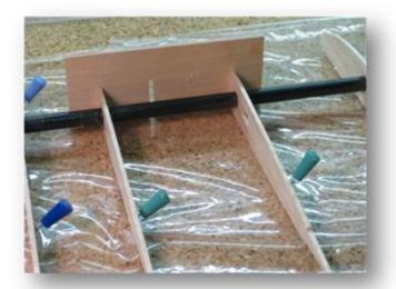
All remaining ribs are aligned now, on the basis of the two middle ribs, by means of the rib comb and stuck together with second adhesive. Note: For all ribs is valid here the larger distance (ca.68 mm)
