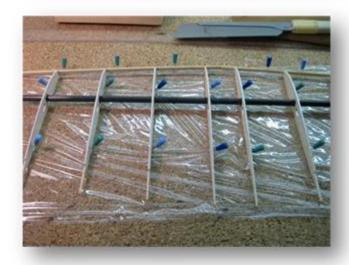
Separate now the 5 mm beech round bar in the center and stick you firmly him as ledge into the recesses with second adhesive.
