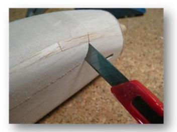
After the trunk was sanded, separate with a sharp measurer carefully the canopy out.
