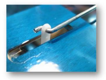
... the other end with that Z-connection is hung up into the servo arm.
