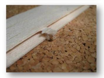
Cut now of the rudder ABOVE a 4 mm off of strips, DOWN a 8 mm of strips.
